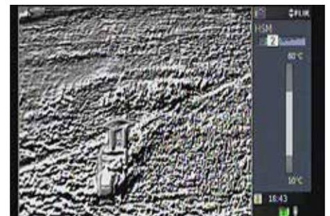
During a UAV test flight, a leaking gas bottle was placed on the ground and the FLIR G300a was able to monitor it very accurately from the air (top: thermal mode, bottom: HSM mode).
