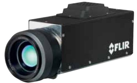
The FLIR G300a optical gas camera contains a cooled Indium Antimonide (InSb) detector that produces thermal images of 320 x 240 pixels.
