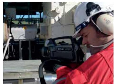
Thanks to optical gas imaging cameras, Inspectahire can easily detect gases in difficult to reach or hazardous locations.
