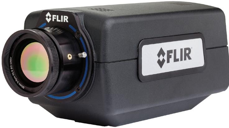
The FLIR A6750 SLS incorporates a cooled Strained Layer Superlattice (SLS) detector that operates in the 7.5 to 10.5  $\mu\text{m}$  waveband, to produce crisp, 640 x 512 pixel thermal imagery. Record high-speed data at up to 4.1 kHz with windowing, and synchronize with other instruments to ensure you never miss any data.
